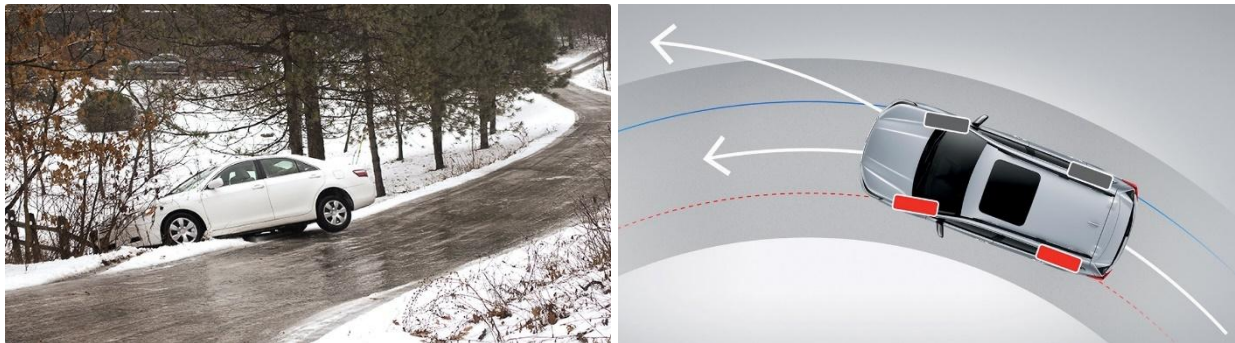
Figure 3. The occurrence of sideslip when the friction between the wheels is different
