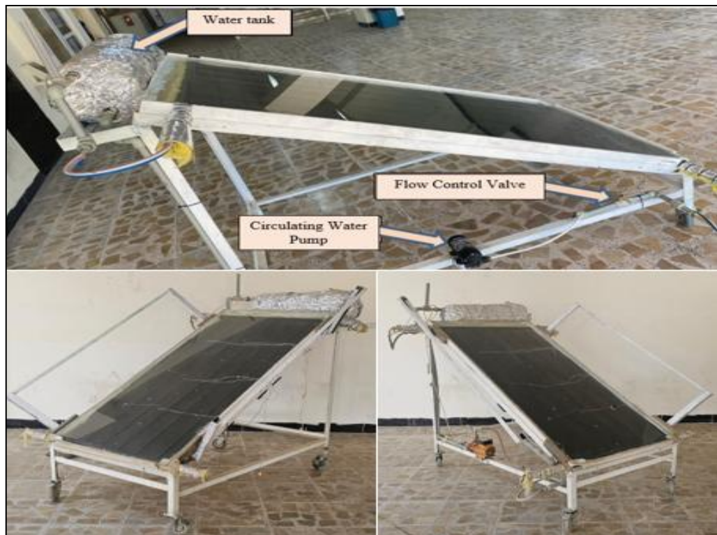
Figure 1: Test Case for Solar Collector Without Reflector After Fabrication and Configuration
