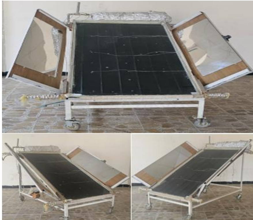
Figure 2: For solar collectors in case of using reflective mirrors
