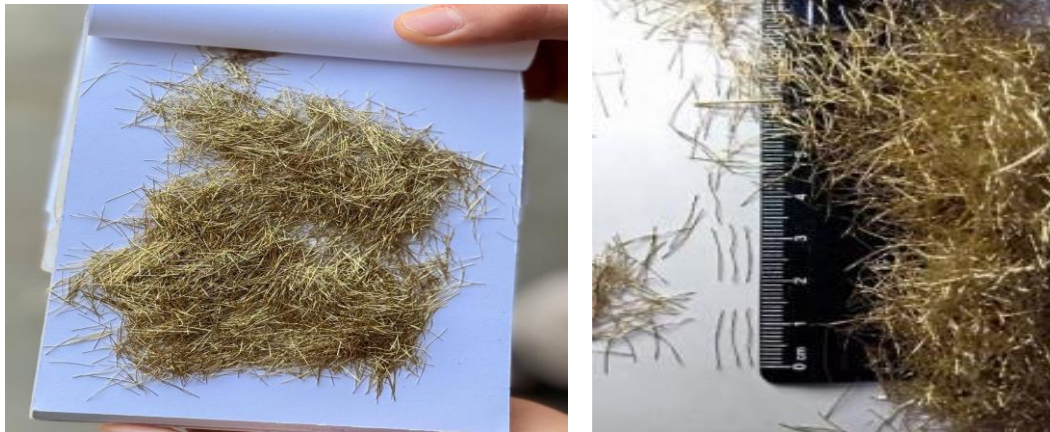
Figure (2): Photo of copper-coated micro steel fiber
